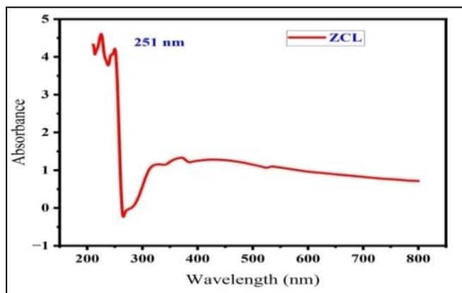
Figure 2: UV-Visible spectrum of ZnO nanoparticles
