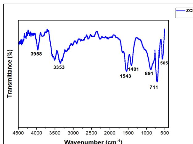
Figure 4: FT-IR spectrum of ZnO NPs
