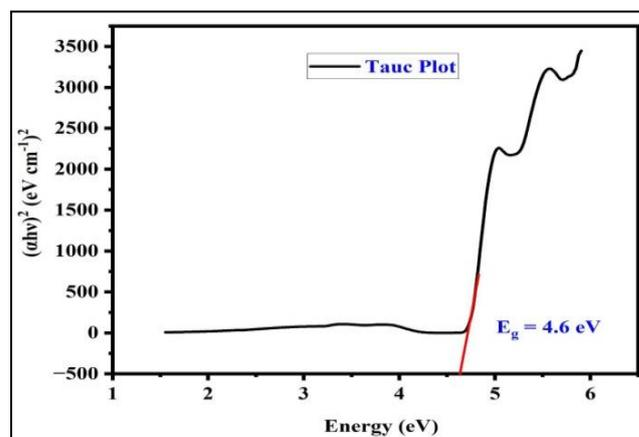
Figure 3: Band gap energy of TCL-ZnO NP and ZCL-ZnO NP
